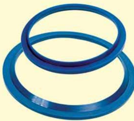
The seals mentioned as Wiper Seal avoid entrance of any kind of dirt and unwished particles in hydraulic system as well as the cylinder. It must consider working condition when choosing wiper seal at hydraulic cylinder. Wiper seals that choose must have scraper characterize if hydraulic cylinder is going to work in dirty and muddy conditions and must have wiper characterized if hydraulic cylinder is not a heavy duty cylinder, if it
